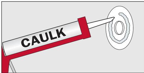
Caulk may be applied to the back of the Dry Seal Pipe Collar when using over grout lines or irregular walls.
