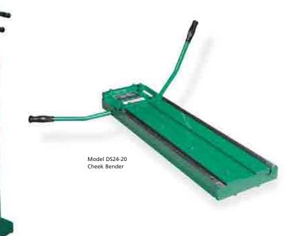
TENNSMITH'S cleat benders are manually operated tools that form uniform drive cleat edges on rectangular ductwork in seconds without set-up or adjustment. The upper handle forms the cleat and the lower handle opens the tool for easy removal of the material. Heavy cast iron and fabricated steel construction provides long life and trouble-free operation. A TENNSMITH cleat bender can save you time and money.
