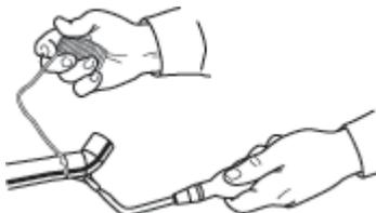
6. Remove excess solder with a small brush or wiping cloth while the solder is plastic.
