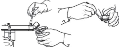
4. Apply flame to the fitting to heat tube and solder cup of fitting until solder melts when placed at joint of tube and fitting.
