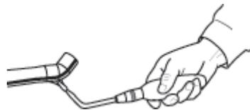
5. Remove flame and feed solder into the joint at one or two points until a ring of solder appears at the end of the fitting. The correct amount of solder is approximately equal to  $1\frac{1}{2}$  the diameter of the fitting...  $\frac{3}{4}$ " (20mm) solder for  $\frac{1}{2}$ " fitting, etc.
