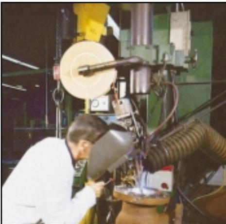
**1** Automatic seal welding of Stellite 6 hardfaced seats.
