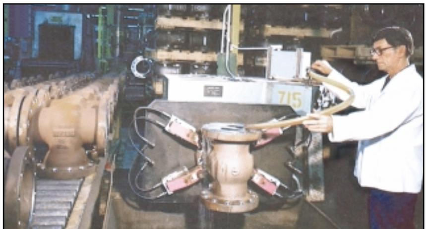
**2** Air-under-water test of the seat's welds.
