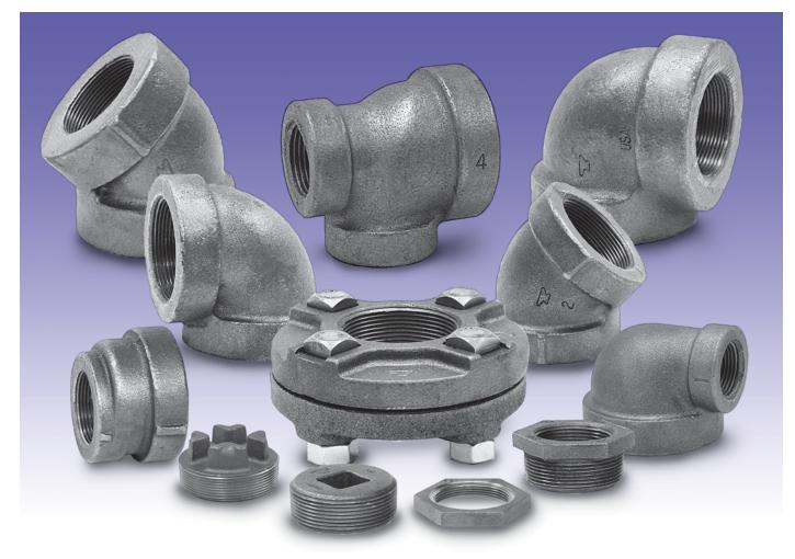
Anvil standard and extra heavy cast iron threaded fittings are manufactured in accordance with ASME-B16.4 (except plugs and bushings, ASME B16.14). Dimensions also conform to Federal Specifications, WW-P-501 (except plugs and bushings WW-P-471).
