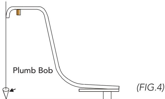
5. Using a plumb bob or level, project front edge of tub lip down to floor surface and make a mark on floor. Repeat several times across front of tub. Draw a straight line at these marks.
