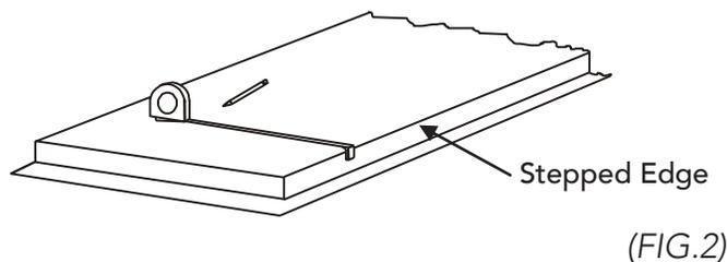
2. Lay apron face-up on flat surface. Hook tape measure on stepped edge of apron near top and mark the adjusted dimension (identified in step 1) near the bottom edge of apron. Repeat this several times across length of the apron. Draw a straight line at the marks on apron. This will be your cut line to custom fit the apron to your installation.
