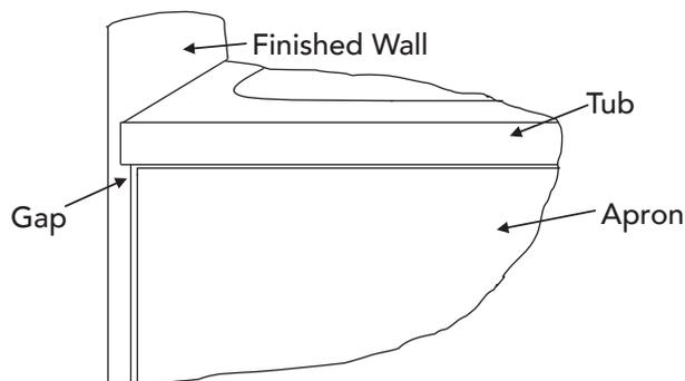
Note: Final installation will leave clearance between both ends of apron and finished wall to allow for future removal.
