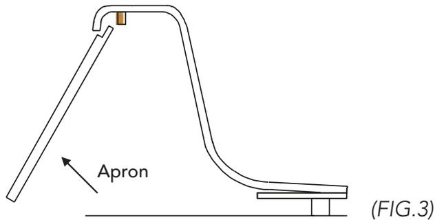
4. Insert the lip of trimmed apron up under tub edge, between the wooden blocks and the front tub lip. Check to see that you have cut the apron to the proper height. Remove apron.
