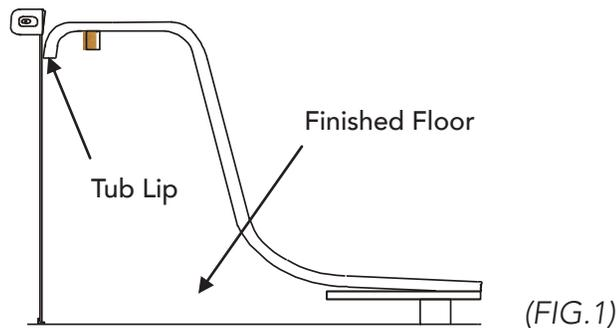
1. With soaking tub or whirlpool in place, measure from the bottom of the tub lip to the finished floor surface. Subtract 1/8" from this dimension for clearance. This adjusted dimension will be used to determine the proper apron height for your installation.
