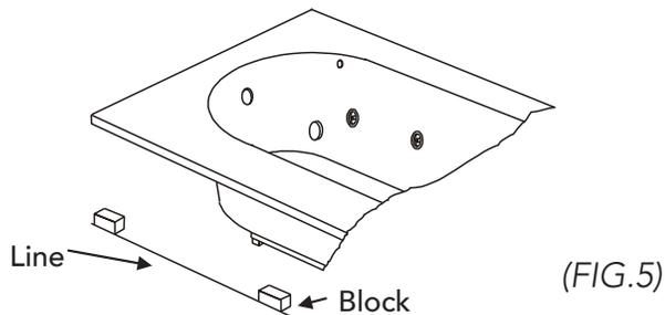
6. Attach at least 3 wooden blocks (not provided), to be used as back-stops, (1"x1" or 2"x2" and at least 6" in length), along the inside of the line drawn in Step 5. Secure blocks with screws or nails if your floor is wood. If your floor is concrete or tiled you will need to use an adhesive to attach the blocks.
