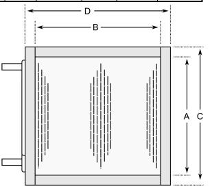
Galvanized steel frame with 1" flange using 18 gauge brackets and 20 gauge sides. Copper waterways using 1/2" O.D. seamless tubes with .017" walls. 500 PSI maximum operating pressure, 2500 PSI ultimate pressure. Aluminum fins are .0045" thick and tubes are expanded into fins for permanent surface bond and maximum heat transfer.
