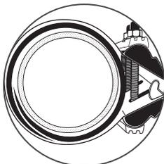
Once the EZ-MAX is positioned around the pipe, re-engage the nut side compression beam over the lug assembly by pushing it downward until it clicks in place TWICE.
