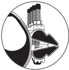
Recharge the line and check for leaks. If any leakage across the seal end is evident, reduce the pressure in the line and increase the labeled torque of the bolts up to 20%.
