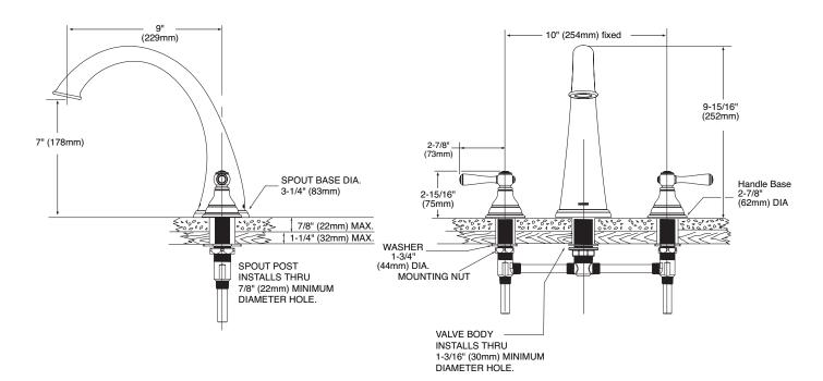
NOTE: THE INSTALLATION SHOWN IS FOR TILE DECKS, THIS VALVE WILL ALSO FIT STEEL, CAST IRON OR PLASTIC DECKS CRITICAL DIMENSIONS
