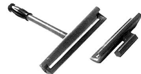
CLEATER Ideal tool to attach cleat to Ductmate 25/35 Flange Joint where space is not a consideration. Use Cleater II in conjunction with 5/8" deep-wall socket, extensions and wrench (not included) to attach cleat to Ductmate 25/35 in hard to reach places.
