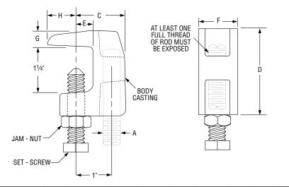
FIG. 93: DIMENSIONS (IN) • LOAD (LBS) • TORQUE (IN-LBS) • WEIGHT (LBS)
