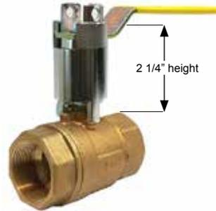
The -XLD extended locking handle is made of robust plated steel and provides additional safety benefits for the user. The handle can be locked in both the open and closed positions. Extension length provides for handle clearance above standard piping insulation thicknesses.
