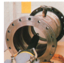
Radiographic inspection checks the integrity of welds.
