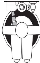
3. When the user steps away from the Object Lock Infrared Sensor, the circuit initiates the flushing cycle to flush the fixture. The Circuit then automatically resets and is ready for the next user.
