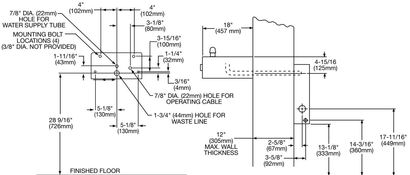
NOTE: ALL DIMENSIONS ARE TAKEN FROM THE FINISHED FLOOR ON THE SIDE OF THE WALL THAT THE FOUNTAIN IS ON.
