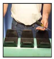
1. Size the casing spacers using charts on appropriate product pages. When opening packaging, make sure you have the correct amount of segments, bolts and nuts for your application.
