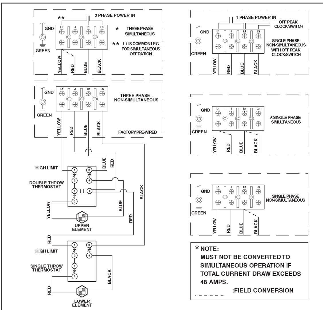
Figure 2. Four-Wire A-8 Circuit for Dual-Element Heater
