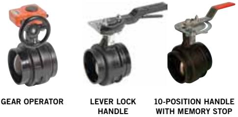
Vic®-300 MasterSeal™ butterfly valves are designed for pressures ranging from full vacuum to 300 psi/2065 kPa and for bi-directional, dead end services to full working pressure. The valve features a patented seat design that assures full 360° sealing. The pressure-enhanced seat compresses to form a larger seating area as the pressure increases. The seat design also contributes to the low breakaway torque capabilities of the MasterSeal valve.
