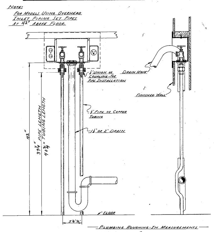
FOR SPACE SAVER WASHING MACHINE SUPPLY AND DRAIN
