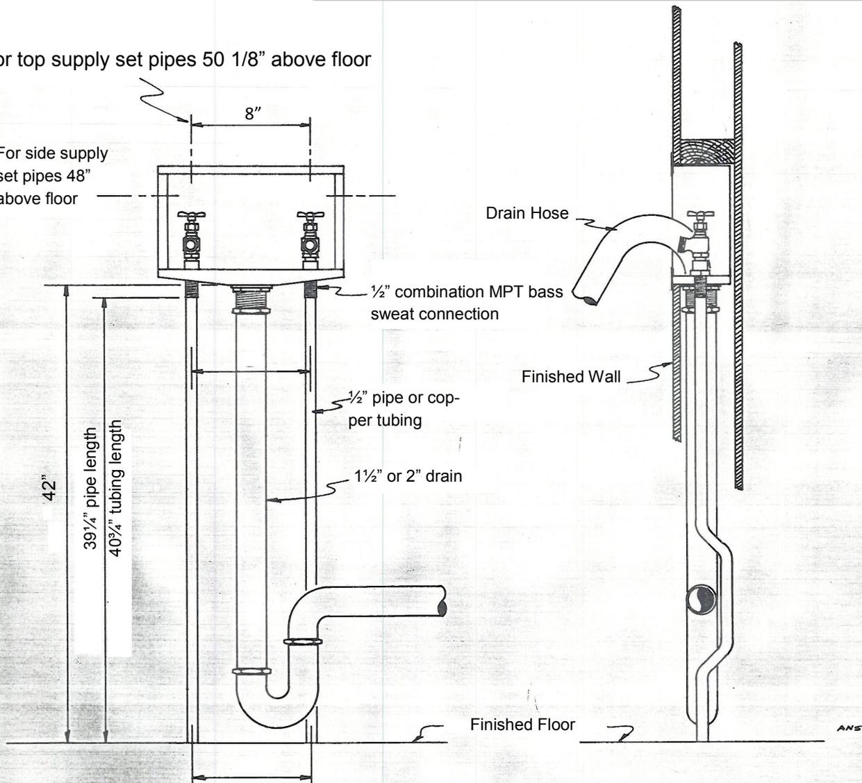
Plumbing rough-in measurements for space saver
