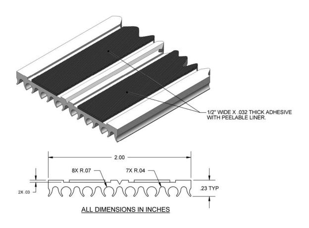
The HOLDRITE<sup>®</sup> Silencer™ #271 is an engineered sound isolation lining with many versatile applications for use in minimizing noise transfer with plumbing and piping systems. This 2" wide strip comes in 25' rolls and can easily be cut down the center at 1" width. The self adhesive strips provide grip to piping or hangers. Excellent for use in isolating against sound or dissimilar metal contact in hangers or through framing components.
