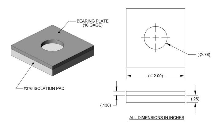
The HOLDRITE® Silencer™ #278 is an engineered sound and vibration isolation pad with a steel bearing plate. Ideal for use in isolating riser clamps and equipment based from noise transfer to the structure.
