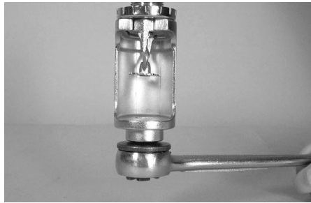
CORRECT ENGAGEMENT FOR MODEL V34 RECESSED WRENCH
