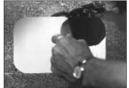
3. Insert door into opening at an angle and tighten knobs.
