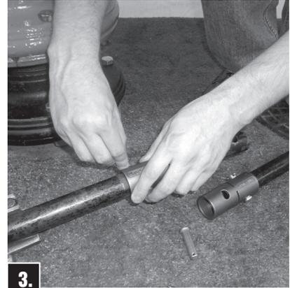
**3.** Place Extension Stem and Extension Coupling on Lower Stem and retain it with stainless steel Clevis Pin and stainless steel Cotter Pin.
