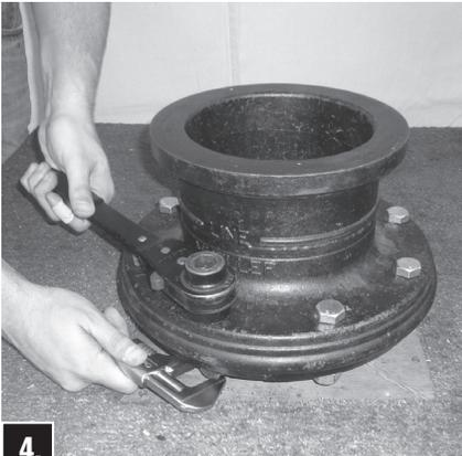
**4.** Attach Extension Barrel to Lower Barrel with solid Flange halves (without groove) and Bolts, being sure O-ring is in place.
