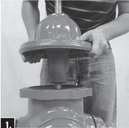
**1.** Remove Hold-Down Nut Operating Nut and Anti-Friction Washer from Bonnet. Lubricate Brass Sleeve and slide over threaded stem to prevent O-ring damage. Unbolt and remove Bonnet. Remove Brass Sleeve.
