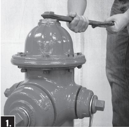
**1.** Remove Hold-Down Nut, Anti-Friction Washer and Operating Nut from Bonnet. Lubricate outside of Brass Sleeve and slide over threaded stem end to prevent O-ring damage. Unbolt Bonnet from Upper Barrel and remove. Remove Brass Sleeve.
