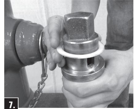
**7.** Check Bonnet O-ring\* for proper position and condition. Attach Brass Sleeve to Upper Stem and lubricate outside to protect O-ring Seals from thread damage. Place Bonnet onto Upper Barrel and assemble Bonnet Bolts only hand-tight. Remove Brass Sleeve. Reassemble Operating Nut, Anti-Friction Washer, and Hold-Down Nut (snug-tighten). Be sure O-ring Seals are in good condition at thread shoulder on outside of Hold-Down Nut and on inside where contact is made with Operating Nut.
