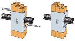
Step 1 Install HSS (HSS2-3 shown) over stud with flanges bent at a 90° angle.
