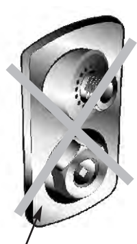
HYDRANT FACEPLATE IN INCORRECT VERTICAL POSITION
