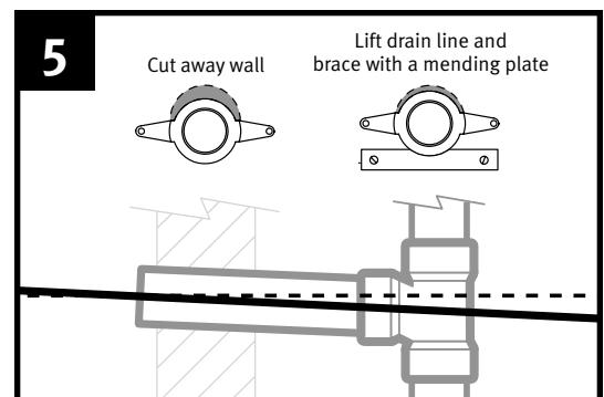
If standing water is present, adjust drain to achieve pitch (code requires 1/4" drop per foot of drain line for proper pitch). Seal wall according to code.
