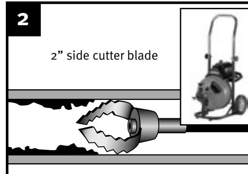
**IMPORTANT:** Use a drain machine to remove build-up inside pipes. Clean 25-35 feet deep then flush with water to remove cutting debris.
