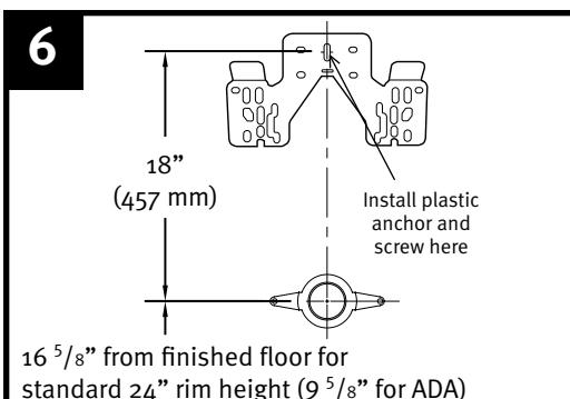
Measure and mark the rough-in. Use a 5/16" masonry bit to drill hole, then install the hanger bracket with one plastic anchor and screw.
