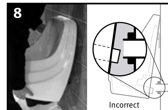
Hang the bowl on the bracket and check tail pipe alignment, then remove the bowl and adjust the bracket as needed.
