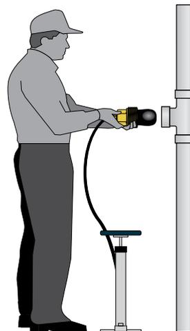
Simply thread into test tee and inflate (for maximum sealing performance, apply thread seal tape to the threads before use).
