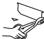
\* **IMPORTANT:** If a rectangular-to-round transition adaptor is used, the bottom corners of the damper will have to be cut to fit, using the tin snips, in order to allow free movement of the damper. Equivalent lengths of duct pieces are based on actual tests and reflect requirements for good venting performance with any hood.
