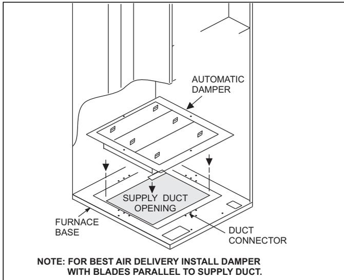
**FIGURE 11:** Anti-Backflow Damper
