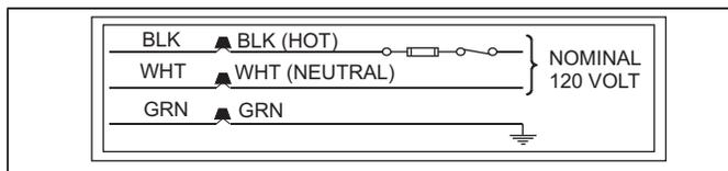
**FIGURE 16:** Line Wiring Connections
