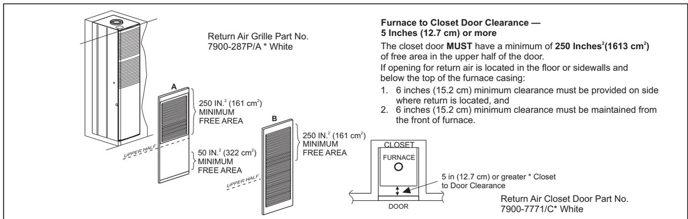
FIGURE 3: Closet To Door Clearance - 5" or Greater
