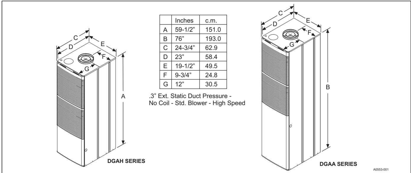
**FIGURE 1:** Furnace Dimensions
