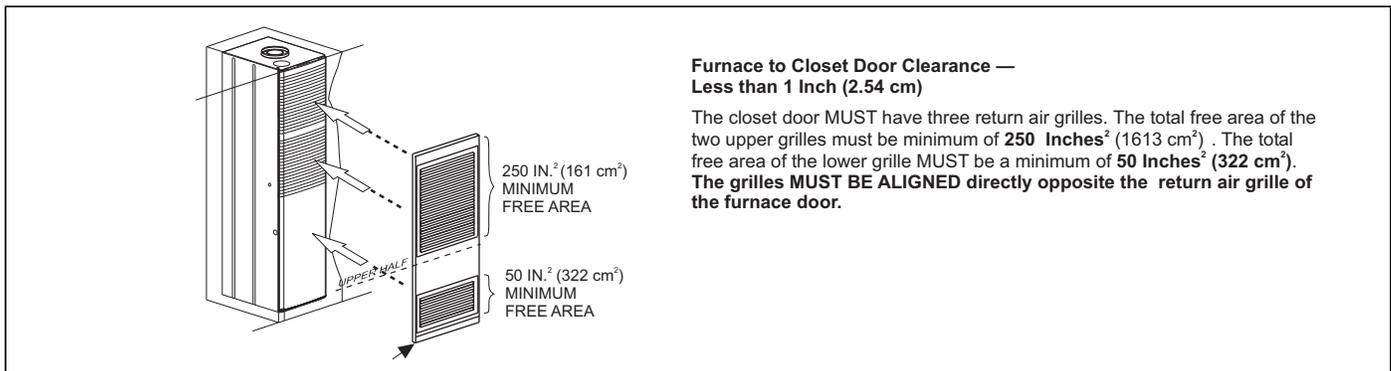
FIGURE 5: Furnace To Closet Door Clearance - Less Than 1"
