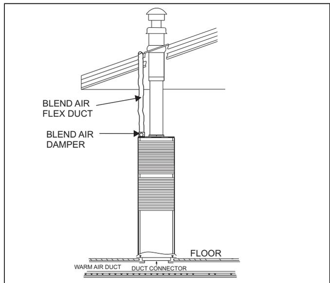
**FIGURE 12:** Floor Installation
