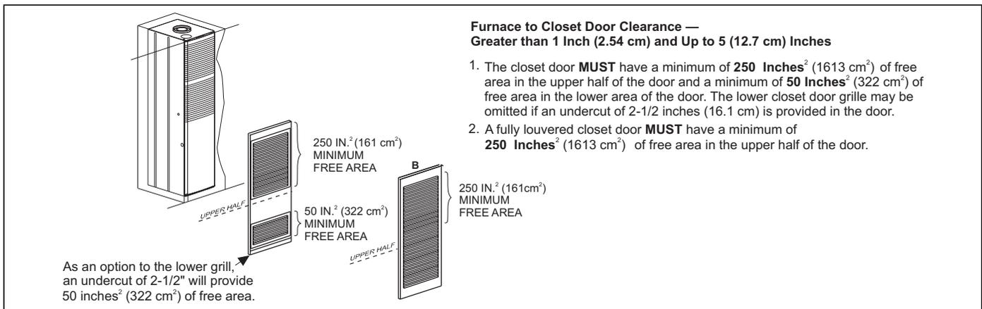
FIGURE 4: Furnace To Closet Door Clearance - 1" To 5"
