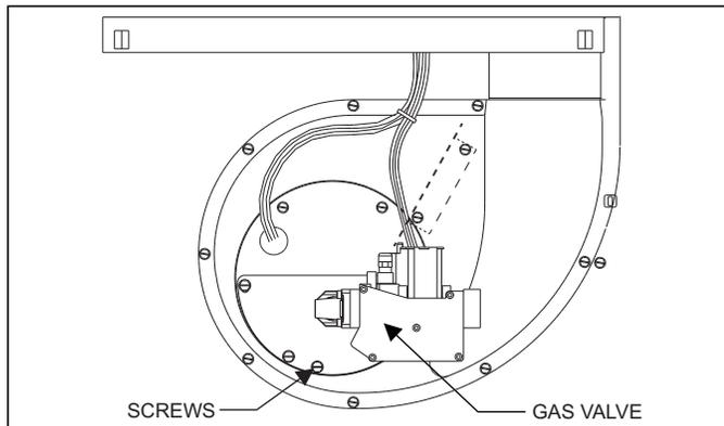
**FIGURE 15:** Burner Assembly
