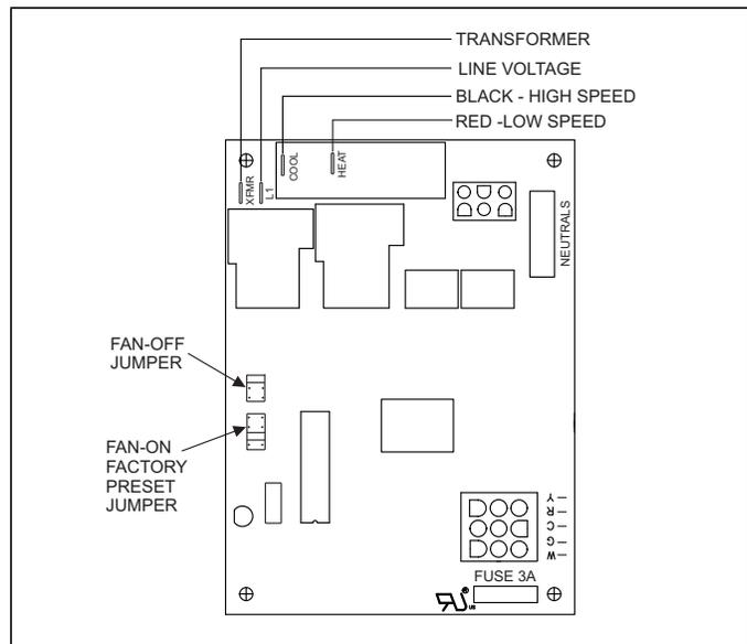
**FIGURE 31:** Furnace Control Board
