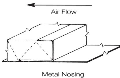
When velocity exceeds 4000 FPM use metal nosing on every leading edge. Nosing may be formed on duct or be channel or zee attached by screws, rivets or welds.
