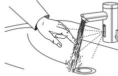
2. As the user's hands enter the beam's effective range, the beam is reflected back into the sensor receiver and activates the solenoid valve allowing water to flow from the faucet. Water will flow until the hands are no longer sensed or until the faucet reaches its automatic time out limit setting.
