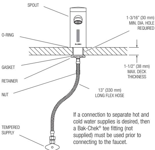
If a connection to separate hot and cold water supplies is desired, then a Bak-Chek® tee fitting (not supplied) must be used prior to connecting to the faucet.
