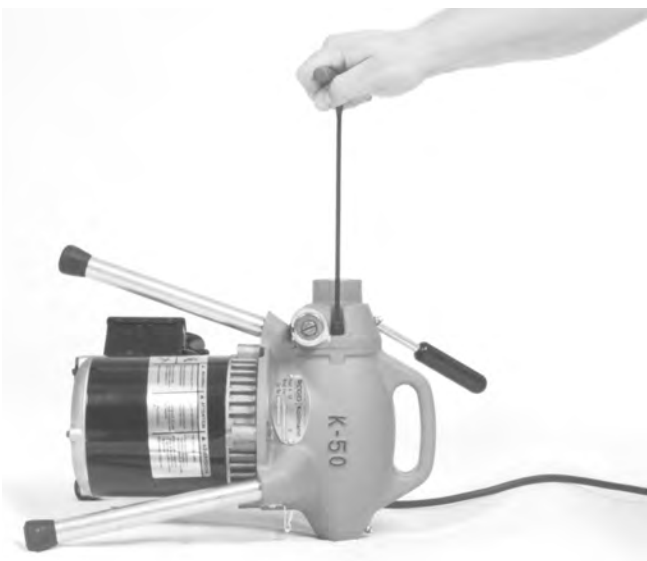
Figure 10 – Retrait des vis Allen
