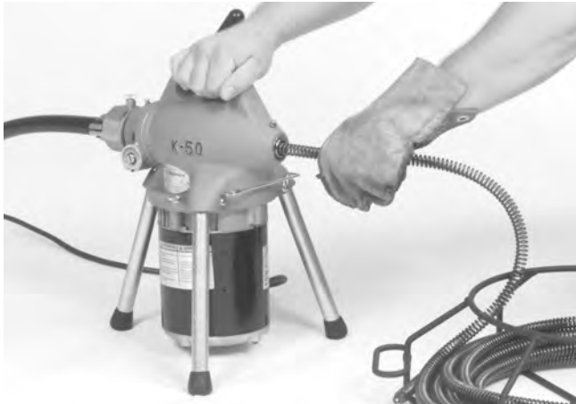
Figure 3 – Inserting Cable Into Front Of Machine
