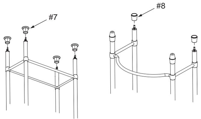
Thread one decorative foot (Item #7) onto the end of each rod until the leading end of the rod is recessed with the foot to a depth of 1/4". **Set the unit upright** and thread one leveling trumpet (Item #8) on the top of the rear legs.
