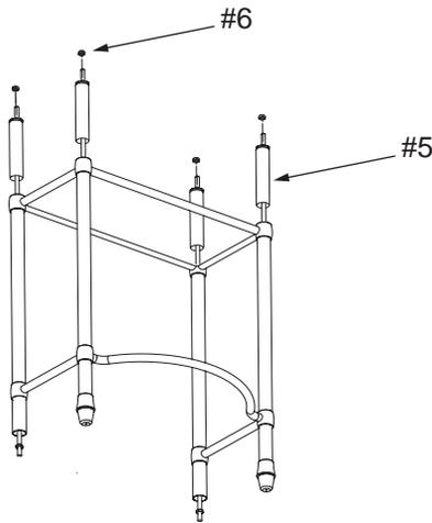
Place a bottom leg tube (Item #5) over each threaded rod such that the closed end of each is nearer to you. Thread one hex nut from the kit (Item #6) onto each rod. Lay the unit down and tighten each of the four legs firmly. Maintain the 5/8" of exposed thread at the top end of the rear legs. Once again, set the unit upside down.
