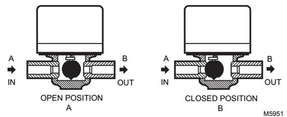
**Fig. 36. V8043 operation for normally closed valve.**
