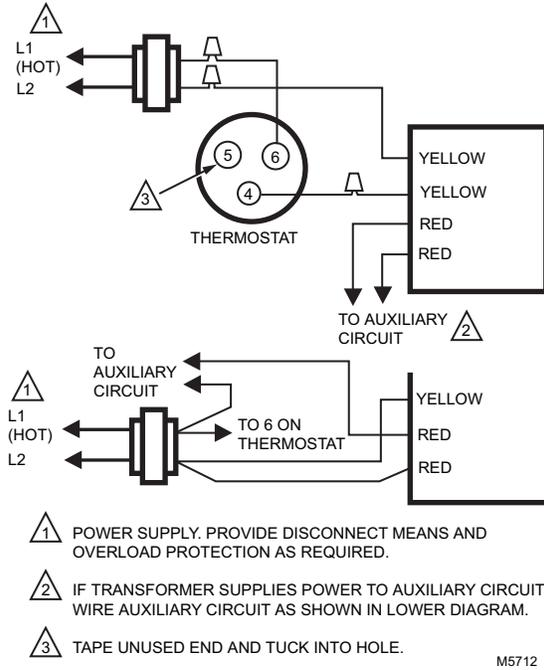
**Fig. 33. Wiring a V8043E to a White-Rodgers System.**
