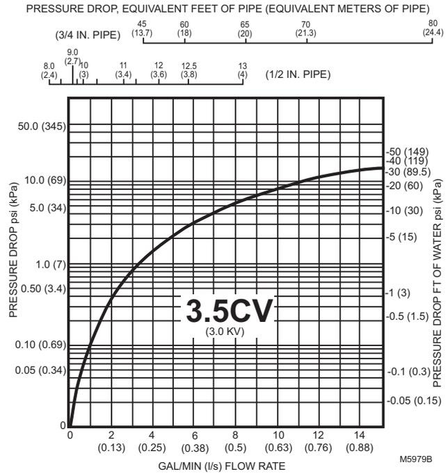
Fig. 5. Flow Characteristics of 3.5 Cv (3.0 kv) valve.
