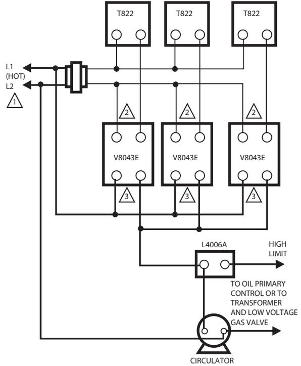
**Fig. 17. T822, V8043E zone hookup for gas or oil. No domestic hot water.**
