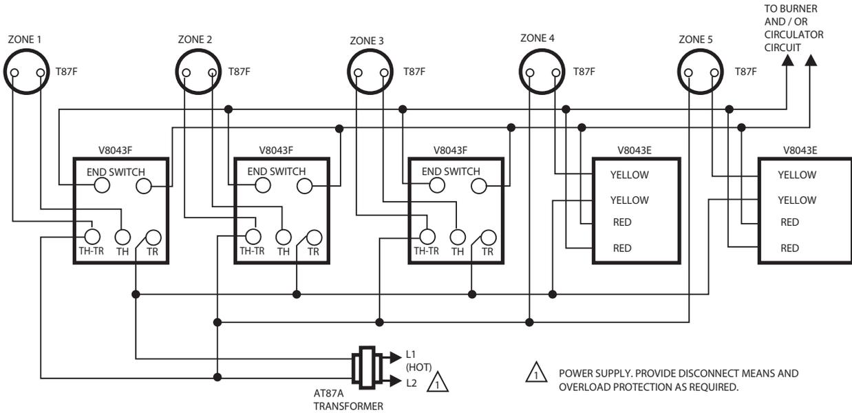
NOTE: IF CODE PERMITS, V8043E AND V8043F CAN BE USED INTERCHANGEABLY WHEN WIRED AS SHOWN.
