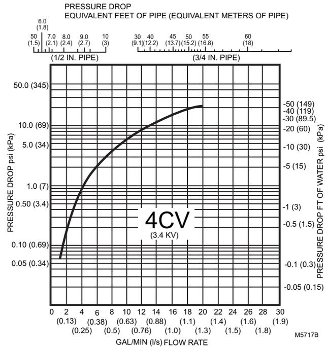
Fig. 6. Flow characteristics of 4 Cv (3.4 kv) valve.
