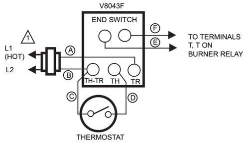
**Fig. 31. Wiring a V8043F to a Flair System (two options). (Wires are identified with letters to correspond with wires on Fig. 29.)**
