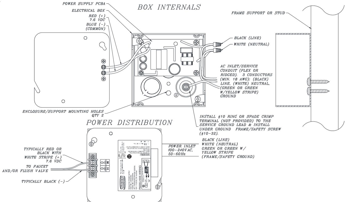
**ENGINEERING SPECIFICATION: ZURN P6000-HW6 Power Converter** - The Hardwired Power Converter is a 7.6 VDC regulated, 2.0A power supply that will operate up to: (8) ZEMS or ZEMS-IS Sensors/Actuators, (8) ZESS Sensors/Solenoids, (8) sensor faucets, or (8) Pint Urinal valves. The unit shown above is integrated into a 4"L x 4"W x 2-1/8"D electrical box. The AC input connections are terminated within the electrical box. The 7.6 VDC output terminals are externally mounted to the cover plate.
