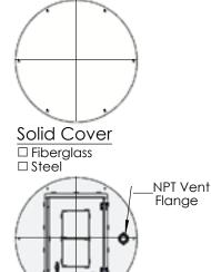
Anti-Floatation Flange-□Fiberglass Encapsulated ASTM A-36 Steel □Round Fiberglass Hinged and Lockable Cover
