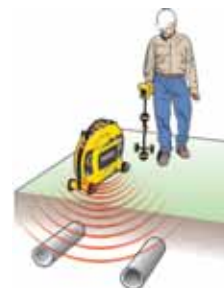
Induce a signal to locate utilities.
