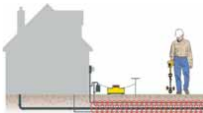
Direct connect to utility lines.
