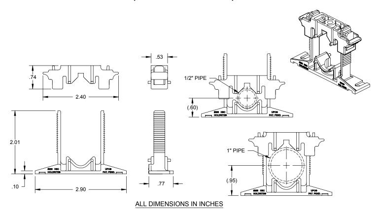
The HOLDRITE® Flame Fighter™ #255-S is a flame and smoke rated variable closure clamp that installs as a standard two hole pipe clamp with one or two screws. Clamp supports up to 1" CTS tubing sizes. Supports Copper, PEX, CPVC tubing, conduit, etc. Material meets ASTM E-84 25/50 and UL94V-0 fire rating.
