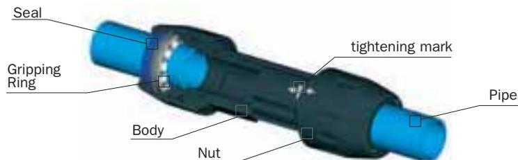
Ø 16,5, Ø 25 and Ø 40 connectors secure instantly to Transair® aluminum pipe. Simply insert the pipe into the connector up to the connector insertion mark.
