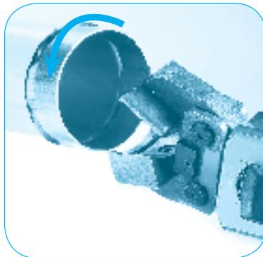
Re-open the two jaws to remove the pipe and rotate the pipe slightly.
