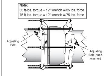
**Step 7** • Check for leaking. Re-tighten the bolts evenly around the pipe as necessary to stop leaking.
