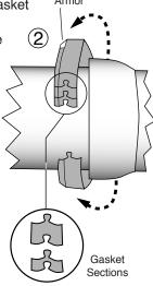
**Step 3** • Align the two armors in the gasket to bridge the gaps at the ends of the casting halves.
