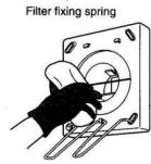
· Be careful not to deform the filter fixing spring.
