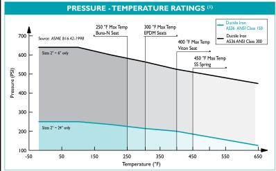
The above chart displays the pressure-temperature ratings for the valve's body material per ASME B16.42-1998. Max temperature limits have been added for seat and spring materials. Sizes 2" through 6" are dual pressure rated for both ANSI Class 150 and 300.
