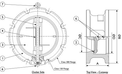
CAD illustration is representative of sizes 2' through 6". Sizes 8" through 24" are not scalloped. Sizes 2" through 6" are designed for <u>dual pressure service</u> (ANSI Class I50 and 300).
