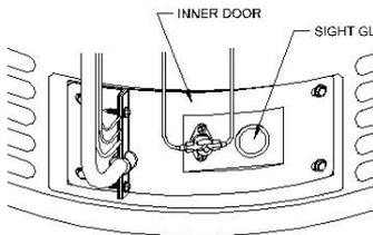
7. Turn the gas control knob clockwise
