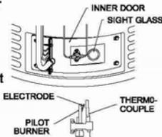
8. Turn the gas control knob counterclockwise
