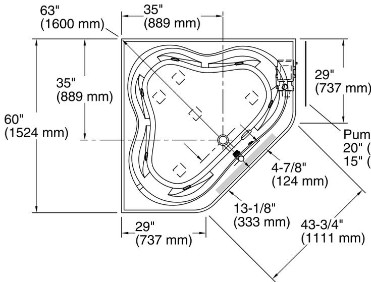
No change in measurements if connected with drain illustrated. (K-11677)
