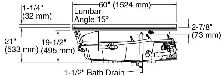
No change in measurements if connected with drain illustrated. (K-11677)
