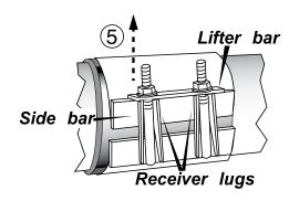
**Step 6** • Tighten all nuts evenly in 15 ft-lb. increments. Keep torques as evenly balanced as possible. Use a wrench with at least a 12" handle.
