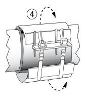
**Note:** If necessary (because of water pressure) Step 4 and Step 5 can be performed beside the pipe break. Slide the clamp over the break after the lifter-bars have been snapped in place.
