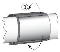
**Step 4** • Back off nuts of shell to the end of the bolt, **DO NOT REMOVE.** Separate clamp and wrap it around the gasket cartridge.
