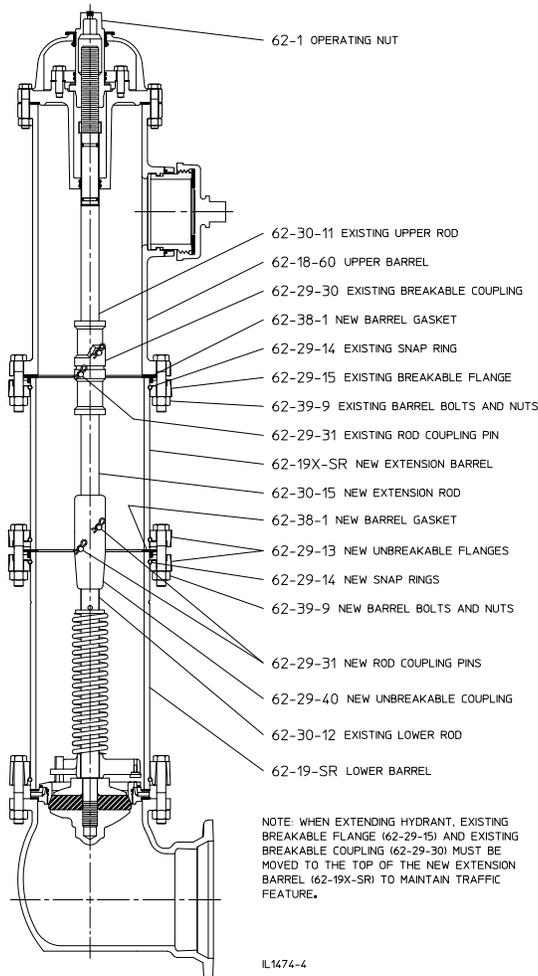
NOTE: The use of extension lengths made by more than one extension kit is not recommended. When combined extension kit and existing trench depth exceeds 9 feet, replace existing lower rod with appropriate length lower rod instead of using rod extension. When combined length exceeds 12 feet, rod guides are recommended for lower rod.
