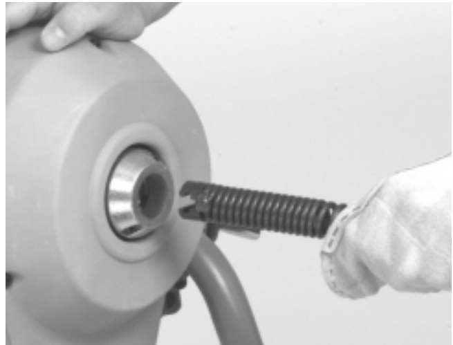
Figure 4 – Inserting Cable Into Front Of Machine
