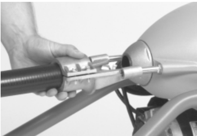
Figure 3 – Rear Guide Hose Attachment
